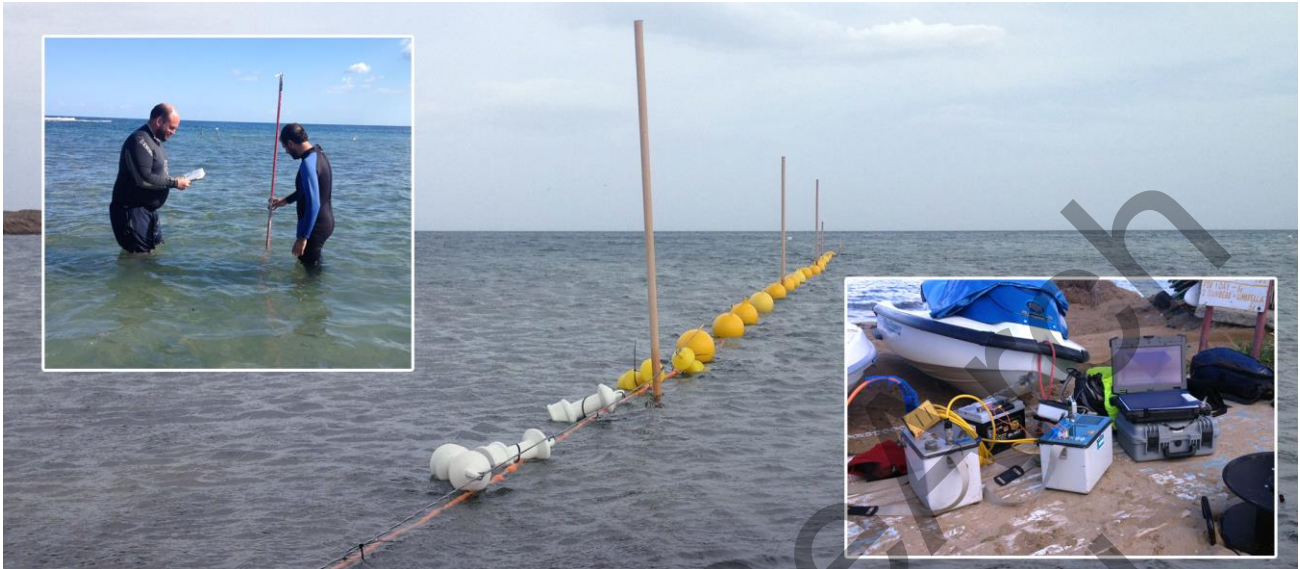
Figure 10. Photo with floating electrodes set up, equipment used (embedded right), water column thickness calculation with a plastic calibrated stick (embedded left).
